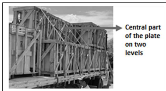
Figure 20: Two levels in the central part of the plate, load leveling.
